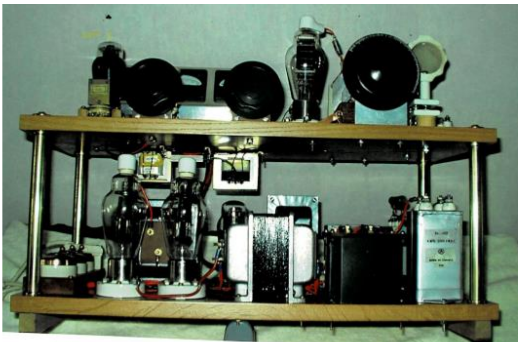
1930s replica CW transmitter
