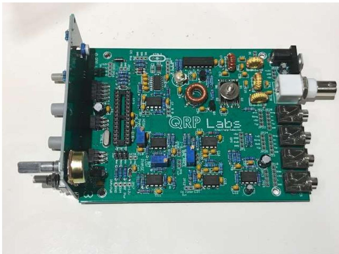
**Figure 2** shows another 3 hour effort and good progress. I encountered a couple issues along the way. Firstly I managed to install the power switch backwards and then, wound the first L1 toroid 3 times before I got it right. And that switch was a bugger of a job to extract too. The solution is to read the instructions before applying solder to the power switch and have a good look at positioning in the board before winding L1-4.
